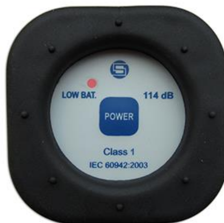
Figure 3. The top view of the SV 33B calibrator with the “LOW BAT.” LED lit
