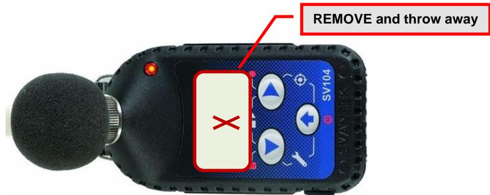
Figure 4-1 Peel off the protection foil and throw it away
