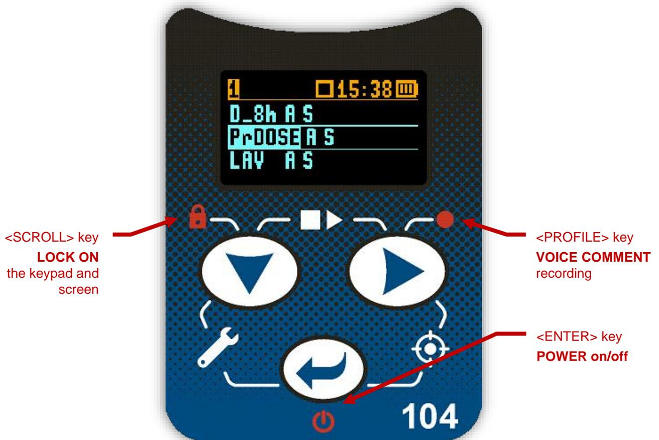
**Figure 3-9** Control keypad on the front panel – alternate key functions
