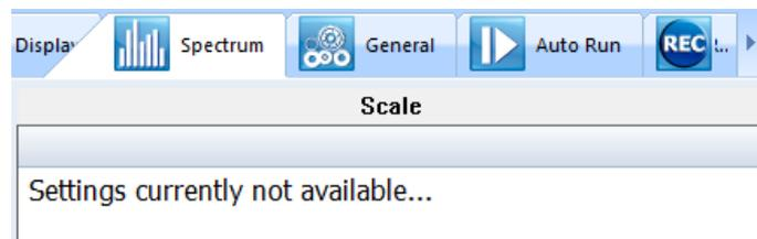
**Figure 5-8** Example of a category of settings unavailable due to some other options in the same setup file being disabled
