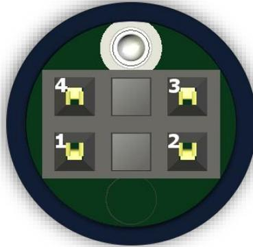
Figure C.5 SV 27 microphone connector (mounting head outer view)
