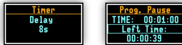
Figure 4-18 Auto-run mode – timer and programmable pause screen
