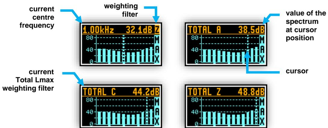
Figure 3-15 1/1 OCTAVE analysis spectrum graph MAX view mode screens
