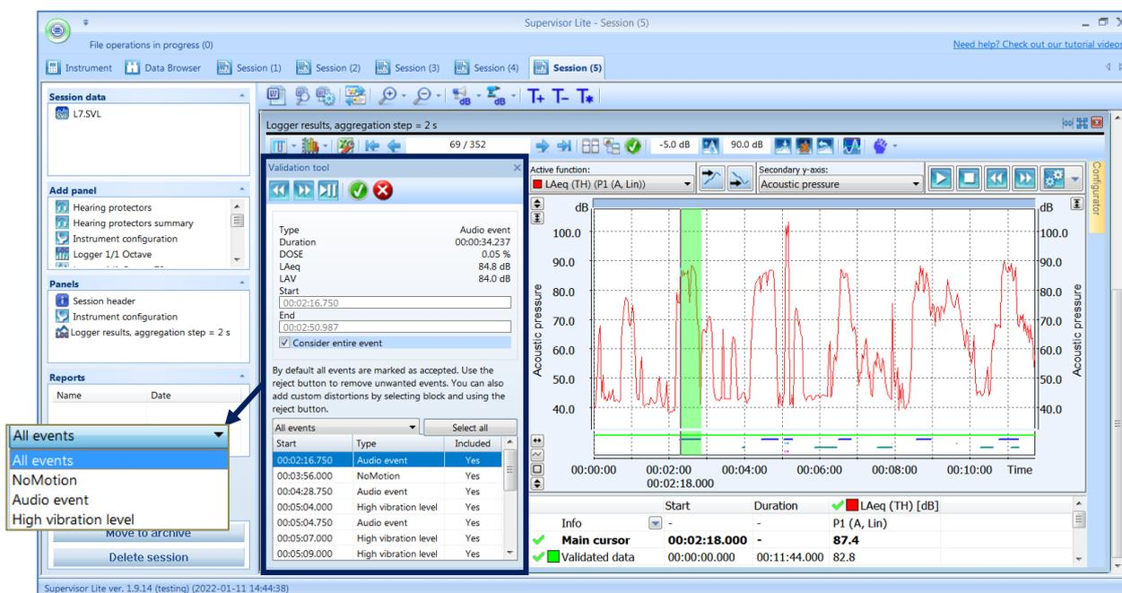
Figure 5-37 Validation tool panel
