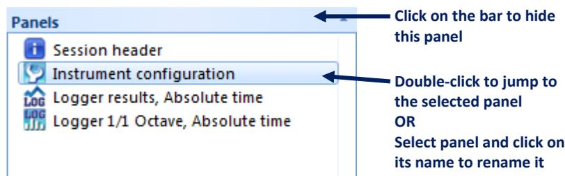
**Figure 5-42** Panels panel, containing a list of panels added to the current session
