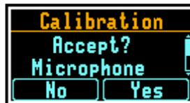
Figure 4-12 Calibration - microphone not in tolerance screen
