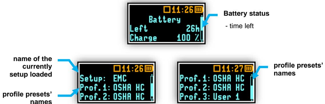
Figure 3-16 INSTRUMENT STATUS view mode screens
