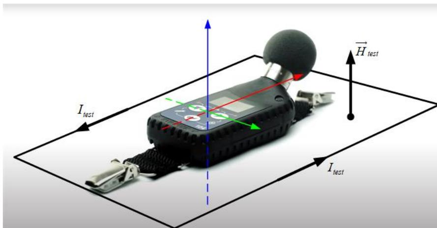
**Figure C.1 SV 104 placed in magnetic field test coil in the direction of maximum response**
