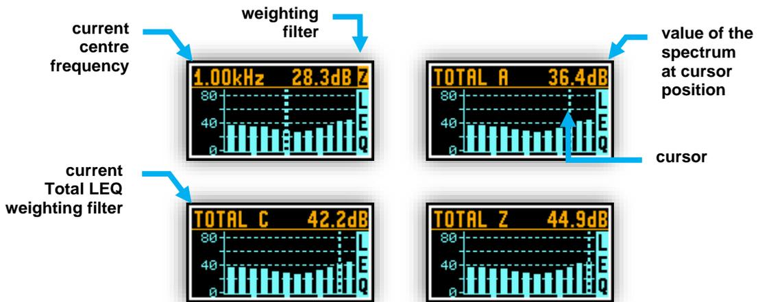
Figure 3-14 1/1 OCTAVE analysis spectrum graph LEQ view mode screens
