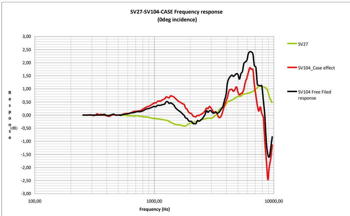
**Figure C.2 SV 104 frequency characteristics**
