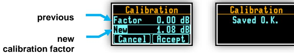
Figure 4-11 Calibration confirmation screen
