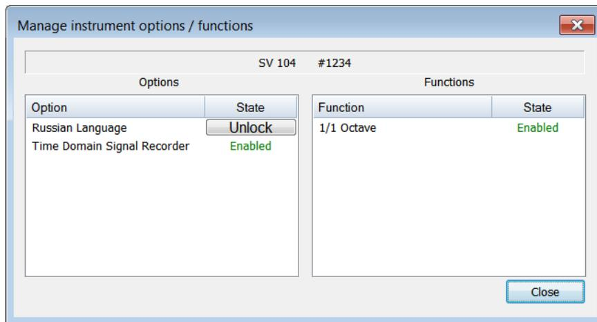
**Figure 5-5** Manage instrument options / functions dialog box
