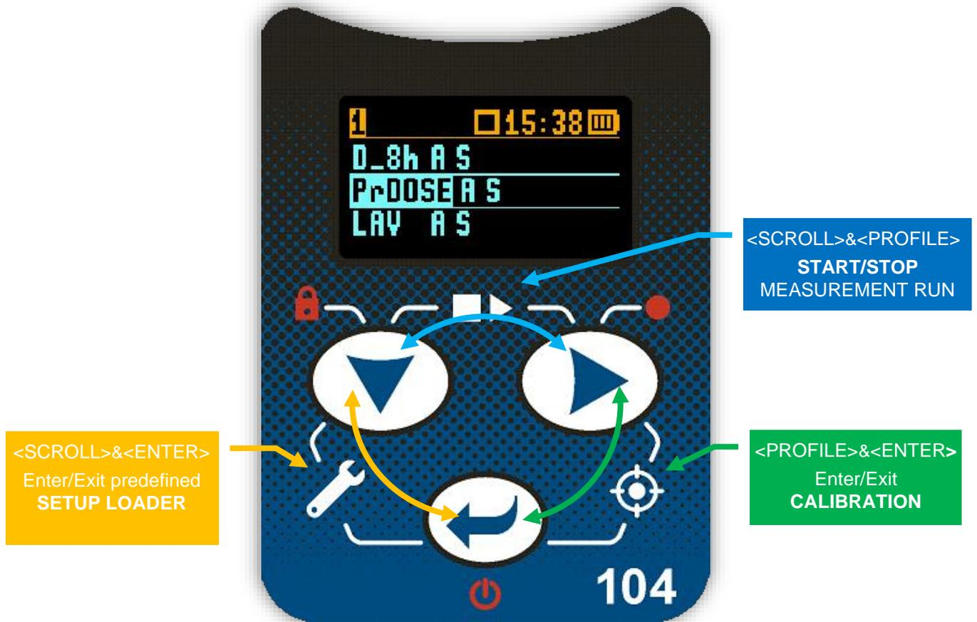
**Figure 3-10** Control keypad on the front panel – alternate combined keys function
