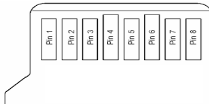
MicroSD contact pad assignment - outer view
