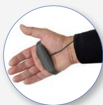
SV 105 Tri-Axial Hand-Arm Vibration Accelerometer
