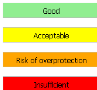
Fig.5-20 Classification of hearing protectors according to L'_A .
