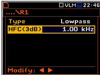
Characteristics of the Lowpass filter with the HFC (3dB) = 1.00 kHz implemented in the instrument
