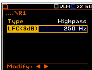
Characteristics of the Highpass filter with the LFC (3dB) = 250 Hz implemented in the instrument
