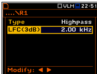
Characteristics of the Highpass filter with the LFC (3dB) = 2.00 kHz implemented in the instrument
