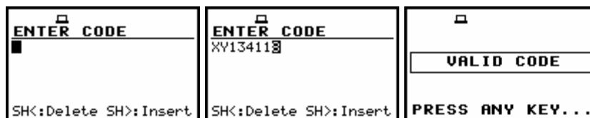
Displays during the entering of the access code to REAL TIME FILTERS
