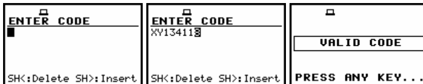
Displays during the entering of the access code to SRT RECORDING, WAVE RECORDING or EVENT RECORDING
