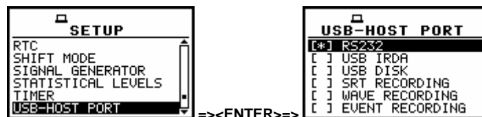
SETUP list with the USB-HOST PORT selected and this window with the activated RS232
