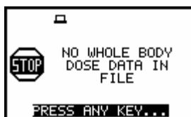
Display after the execution of loading a file without WBV data
