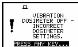
Display in the starting measurements when user selects incorrect filters for HAV/WBV calculations
