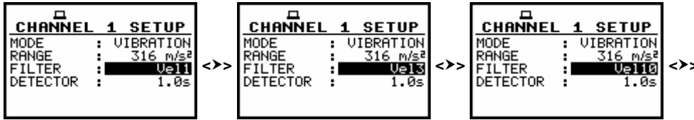
CHANNEL 1 SETUP windows; weighting filters in velocity measurements
