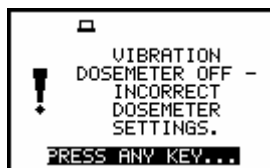
Display in the starting measurements when user selects incorrect filters for HAV/WBV calculations
