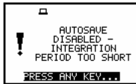
Display, when the INTEGRATION PERIOD is too short for AUTO SAVE option
