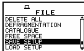
SAVE SETUP text highlighted (displayed inversely) in FILE list
