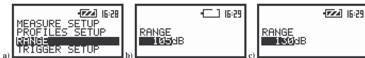
The view of the displays in the INPUT list ( path: MENU / INPUT ) with the RANGE sub-list highlighted (a), the RANGE sub-list when the range is set to 105 dB (b), the RANGE sub-list when the range is set to 130 dB (c)
