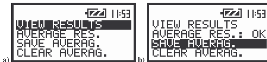
The views of the display (when averaging function is enabled) after the measurement end; (a) screen presents the default situation whereas (b) after setting the last result to averaging process
