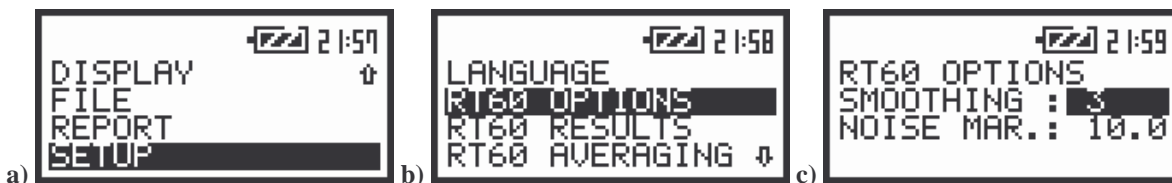
The views of the display in the main list with the SETUP text selected (a), the SETUP list (path: MENU / SETUP) with the RT 60 OPTIONS text highlighted (b), the RT 60 OPTIONS sub-list (path: MENU / SETUP / RT 60 OPTIONS) (c)
