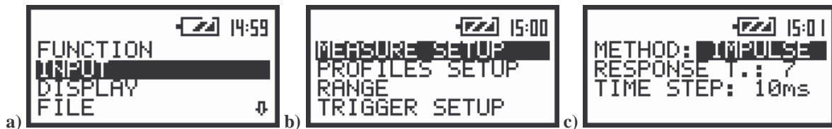
The view of the displays in the main list with the INPUT text selected (a), the INPUT list (path: MENU / INPUT) with the MEASURE SETUP text selected (b), the MEASURE SETUP sub-list (path: MENU / INPUT / MEASURE SETUP) (c)
