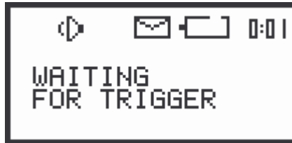
The view of the display when the instrument is waiting for the trigger conditions fulfilment
