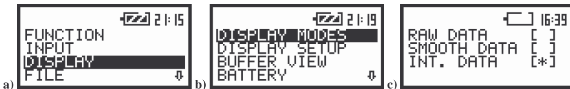
The view of the displays in the main list with the DISPLAY text selected (a), the DISPLAY list (path: MENU / DISPLAY) with the DISPLAY MODES text highlighted (b), the DISPLAY MODES sub-list (path: MENU / DISPLAY / DISPLAY MODES) (c)
