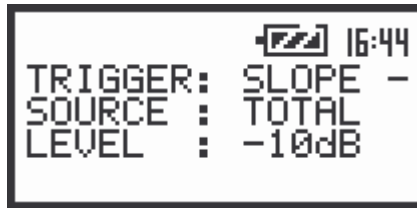
The view of the display in the TRIGGER SETUP sub-list (path: MENU / INPUT / TRIGGER SETUP) for the DECAY method
