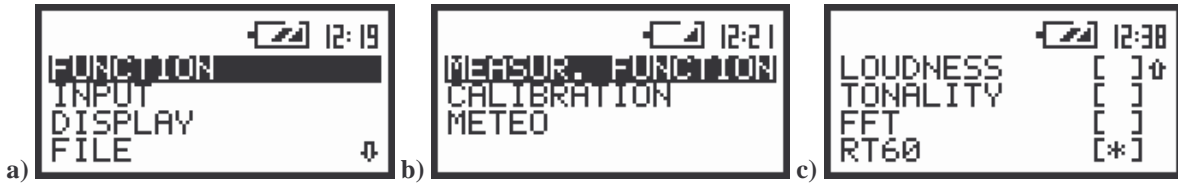
The view of the SVAN 945A displays in the main list with the FUNCTION text selected (a), the FUNCTION list (path: MENU / FUNCTION / MEASUR. FUNCTION) opened with the MEASUR. FUNCTION text selected (b), RT 60 analysis mode selected in MEASUR. FUNCTION sub-list (c)
