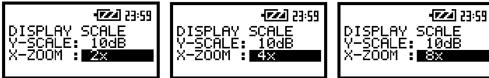
The view of the screens with the possible values of the horizontal axis in PLOT and SPECTRUM presentations
