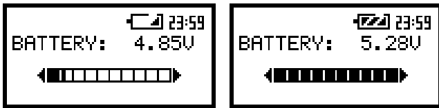
The view of the screens with the BATTERY position when the external supplier is not connected
