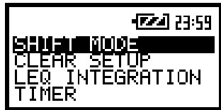
The view of the screen in the SETUP list with the SHIFT MODE sub-list selected
