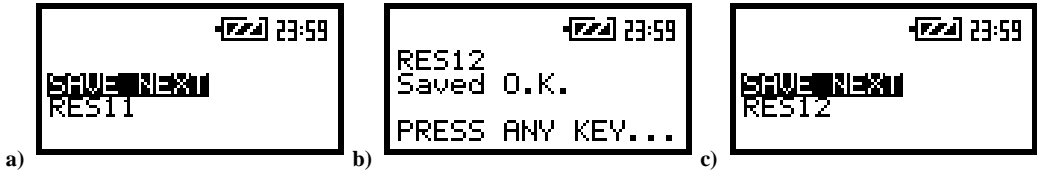
The screens with the SAVE NEXT function (a); after saving the file with the increased name (b) and after repeated enter to the SAVE NEXT function (c)
