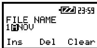
The view of the screen during the process of setting the character in the edited name
