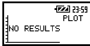
The view of the screen in the PLOT mode when there is nothing in the buffer to be displayed
