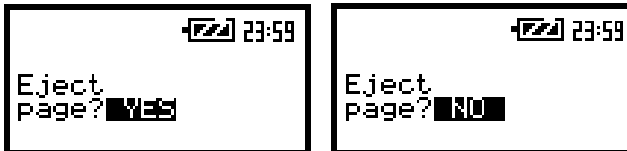
The view of the screens after printing with the confirmation request of the paper ejection
