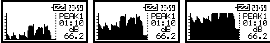
The view of the screens in the PLOT presentation mode with the shifted axes
