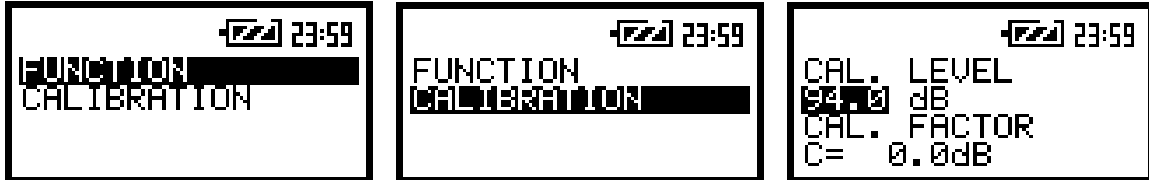
The view of the screens with the FUNCTION list and after entering the CALIBRATION sub-list
