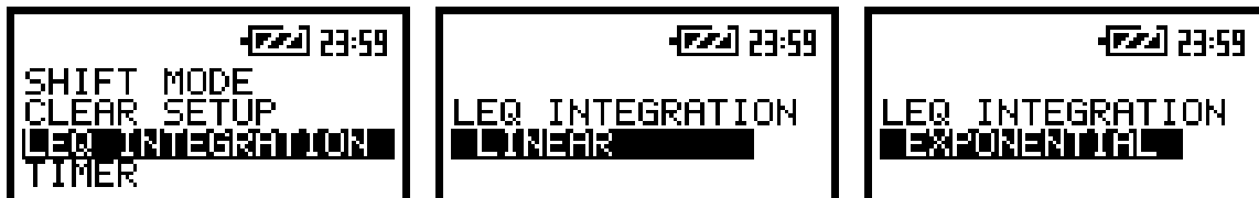
The view of the screens in the SETUP list (a) and with the possible options of LEQ INTEGRATION position (b), (c)
