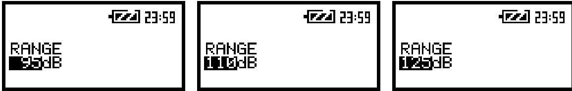
The view of the screens with the RANGE position in 1/3 OCTAVE analysis mode
