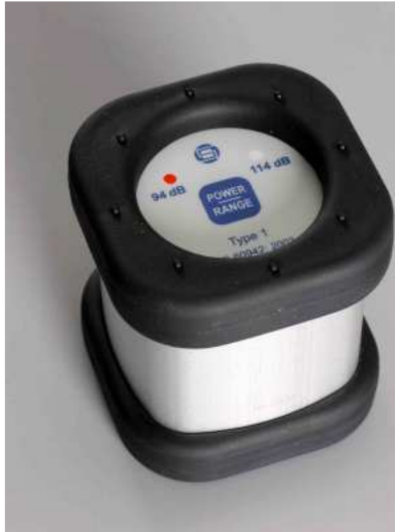
Picture 4. The top view of the SV 30A calibrator with one burning diode
