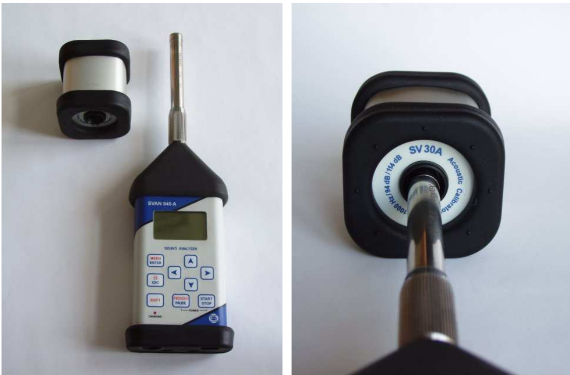
Picture 2. Calibration of the SVAN 945A sound level meter with a \frac{1}{2} " measurement microphone
