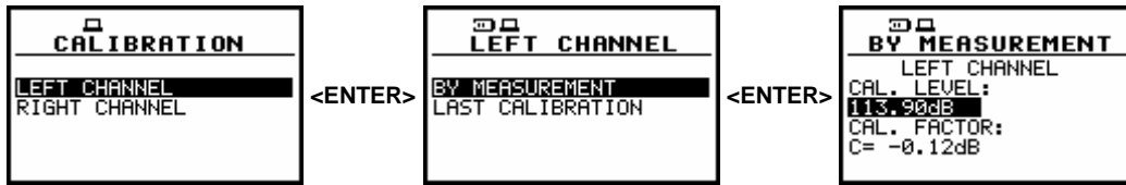
CALIBRATION window with LEFT CHANNEL text selected; BY MEASUREMENT text selected and BY MEASUREMENT window opened
