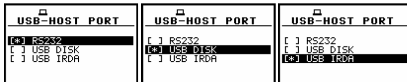
View of the display in the USB-HOST PORT
