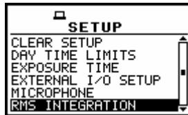
Displays in the SETUP list with the RMS INTEGRATION text highlighted (displayed inversely)
