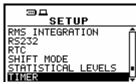
View of the display in the SETUP list, the TIMER text highlighted (displayed inversely)
