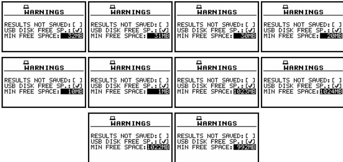
View of the displays in the WARNINGS sub-list; MIN FREE SPACE selection
