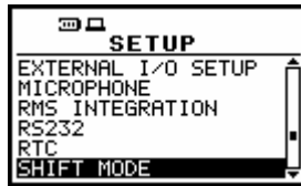
View of the display in the SETUP list, the SHIFT MODE text highlighted (displayed inversely)
