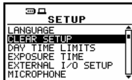
View of the display in the SETUP list, the CLEAR SETUP text highlighted (displayed inversely)
