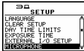
View of the display in the SETUP list, the MICROPHONE text highlighted (displayed inversely)
