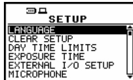
View of the display in the SETUP list, the LANGUAGE text highlighted (displayed inversely)
