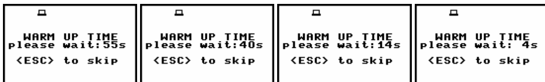
Counting down during the warming up of the instrument after switching it on
