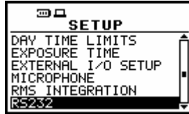
View of the display in the SETUP list, the RS232 text highlighted (displayed inversely)
