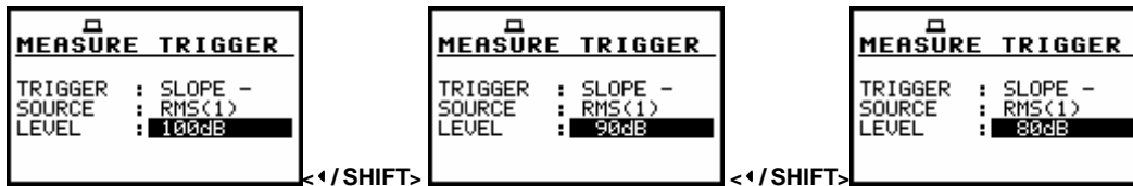
MEASURE TRIGGER window with the LEVEL selection in the SLOPE - mode (10 dB step down)
