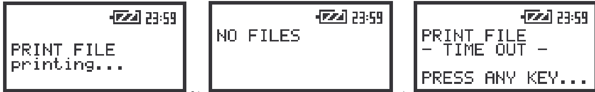
a) b) c) The view of the display during the proper execution of the PRINT FILE operation (a) and in the case when there is something wrong (b, c)
