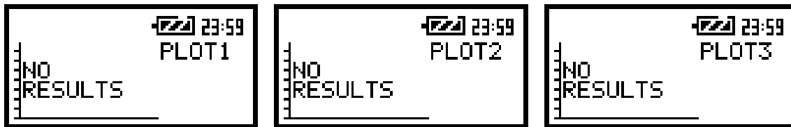
The view of the display in the PLOT mode when there is nothing in the buffer to be displayed
