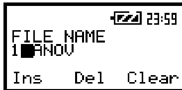
The view of the display after pressing the <INPUT> (Ins) push-button
