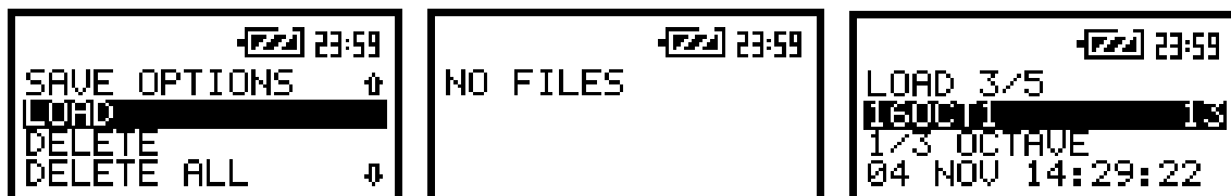
The view of the displays during the execution of the LOAD operation
