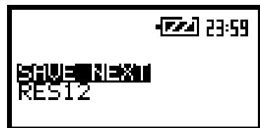
The displays with the SAVE NEXT function (a); after saving the file with the increased name (b) and after repeated enter to the SAVE NEXT function (c)
