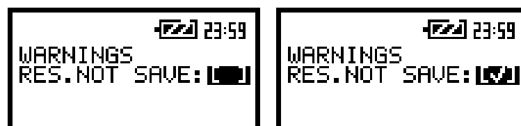
The view of the displays in the WARNINGS window; the selection of the RES.NOT SAVE option
