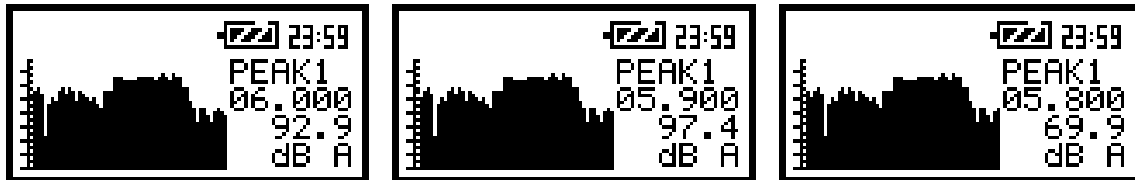
The view of the displays with the selected file from the buffer; the scrolling to the right
