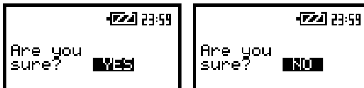
The view of the displays during the execution of the DELETED ALL operation
