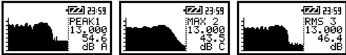
The display views with the selected file from the buffer; the change of the profile after pressing <ENTER>
