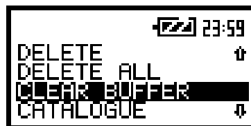
The view of the display in the FILE window with the CLEAR BUFFER window selected
