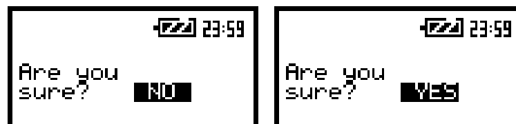
The view of the displays during the execution of the CLEAR BUFFER operation
