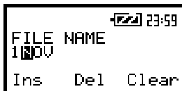
The view of the display after pressing the <DISPLAY> (Del) push-button
