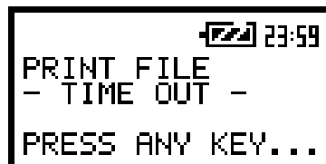
The view of the display during the file printing when there is no data transfer
