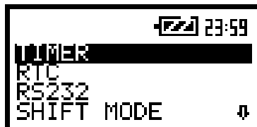
The view of the display in the SETUP window with the TIMER text selected
