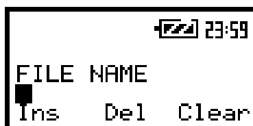
The view of the display after pressing the <FILE> (Clear) push-button
